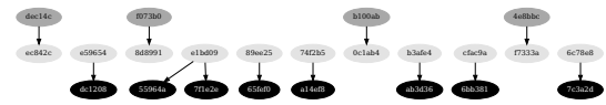
Figure 6: The transaction graph of the Chipmixer experiment. Gray and black nodes are our input and output transactions, respectively. Transactions in light gray nodes generate anonymity sets.
